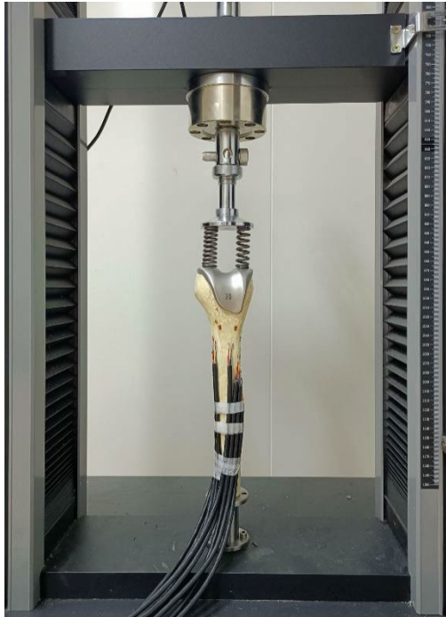
Fig a. Strain test of the synthetic femur under compressive load.
