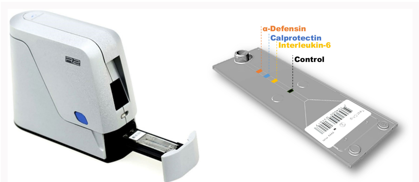
Fig. 1 Analyzer and microfluidic test chip used in this study (for details refer to “Methods”).
