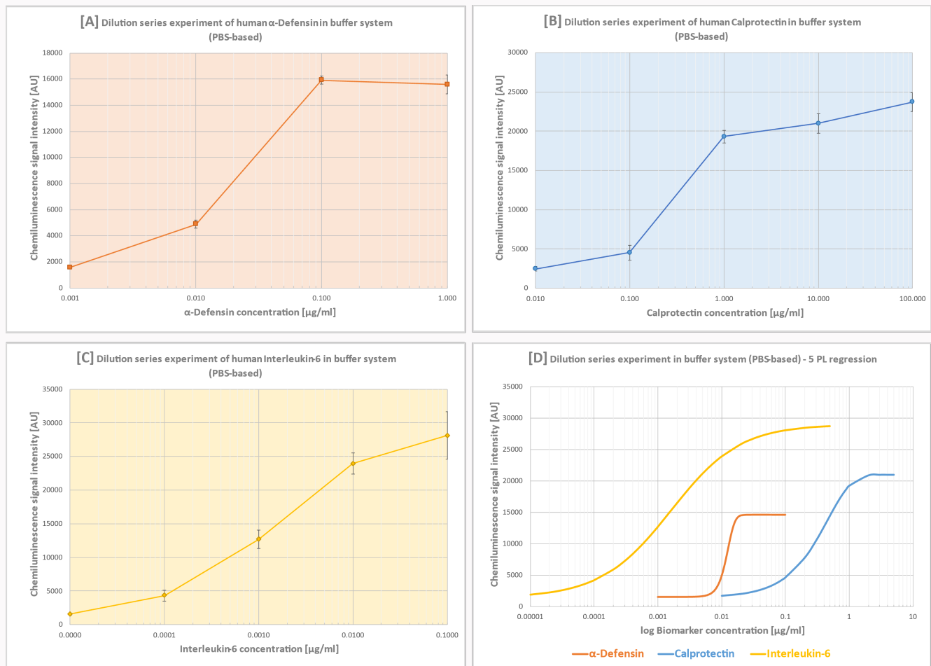
Fig. 3 Buffer-based dilution series experiment for human alpha-defensin, calprotectin, and interleukin-6 (IL-6) diluted using GENSPEED washing solution measured with multiplex GENSPEED test chips. The figure displays the chemiluminescent signal intensities (AU) across various biomarker concentrations. The data represent mean values from three measurements: a) alpha-defensin; b) calprotectin; c) IL-6; and d) five parameters logistic (PL) regression. PBS, phosphate-buffered saline.
